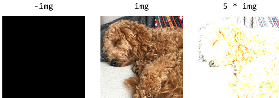
Figure 6.10: Negation and scalar multiplication of an image
