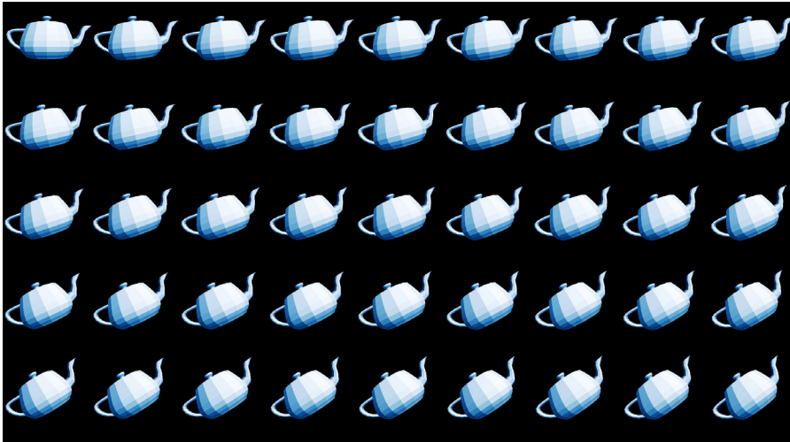
Figure 4.3: Rotating the teapot by 1^\circ at a time, 45 times in a row, beginning with the upper left-hand corner
