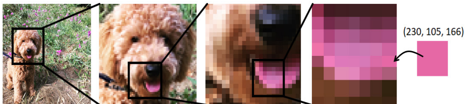
Figure 6.8: Zooming in on a picture of my dog, Melba, until we can pick out one pixel with red, green, and blue content (230, 105, 166, respectively)
