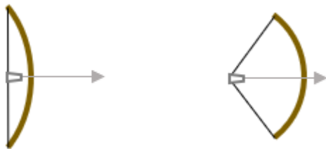
Figure 11.3: On the left, the bow has no potential energy. On the right, it has a lot of potential energy, ready to be spent to put the arrow in motion.
