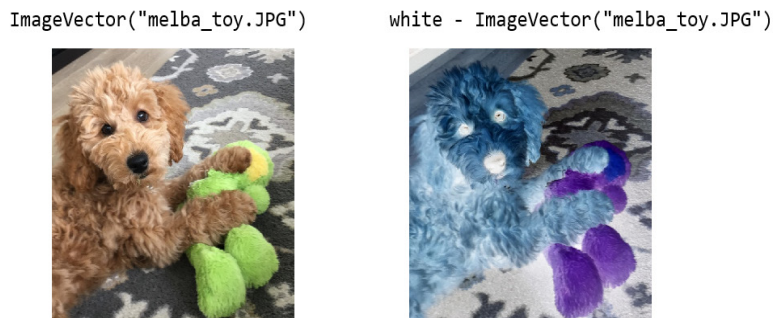
Figure 6.11: Reversing the color of an image by subtracting it from a plain, white image
