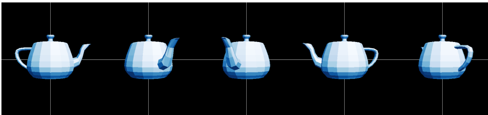
Figure 5.4: The teapot is transformed by a new matrix in every frame, depending on the elapsed time when the frame is drawn.
