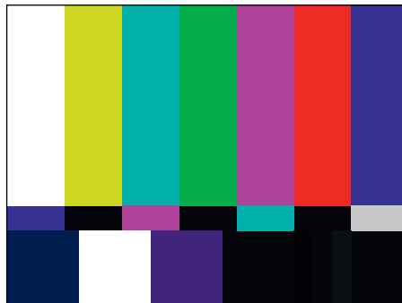
Figure 36.1 The SMPTE EG 1 SD colourbar test signal is represented here as an image; however, it is standardized as a signal in the R'G'B' domain. Its colour interpretation depends upon the primary chromaticities in use. The corresponding Y'C_B C_R or Y'P_B P_R waveforms depend upon luma coefficients and scaling.
